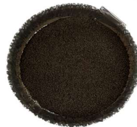
Hydrochar H180°C 30 min. 1:10 ratio
