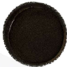
Hydrochar H180°C 30 min. 1:10 ratio
